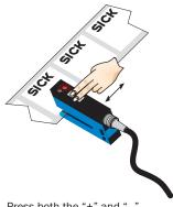
Press both the "+" and "-" buttons together, hold > 1 s and than release the teach-in buttons. The red LED flashes.
