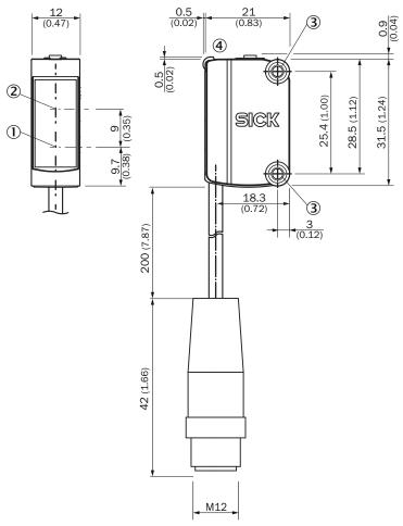
① Center of optical axis, sender
